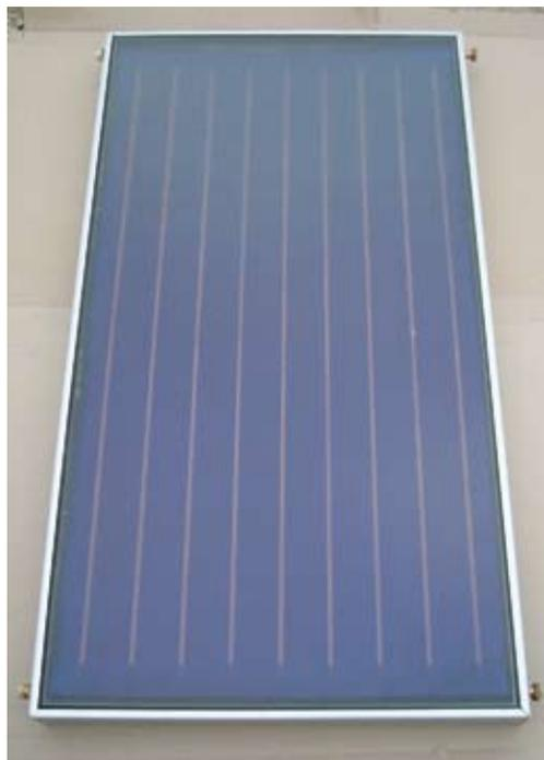
Solex solar panels are high quality traditional flat plate solar collector panels. They have Sunselect blue selective copper absorbers, ultrasonically welded 10mm riser pipes, prismatic solar glass, and aluminium profile casing and backing. Straight through 22mm diameter headers provide good flow rates, and enable easy fitting of multiple panels.
